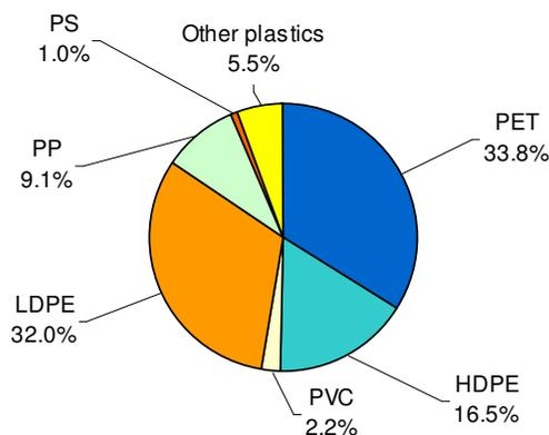
**Figure 5-19 Composition of recovered plastics (by weight), SA 2006**
