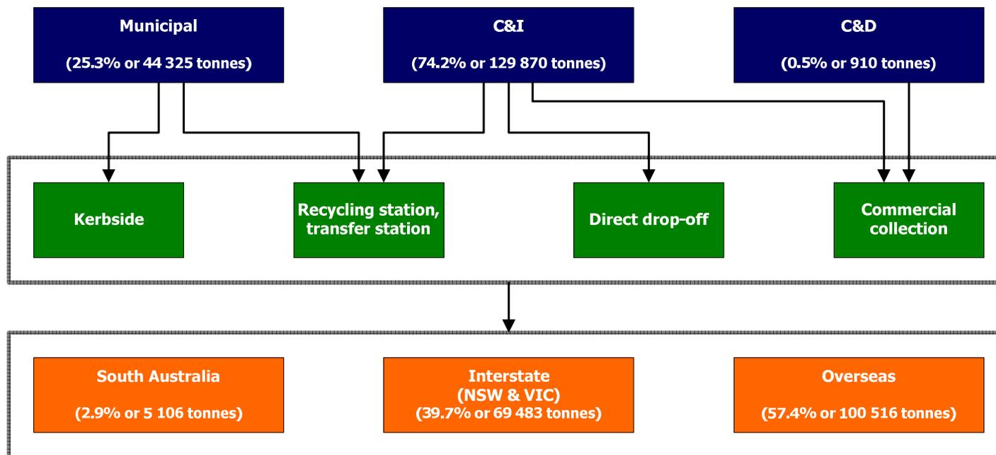
Figure 4-17 Flow of paper & cardboard reprocessing, SA 2006-07
