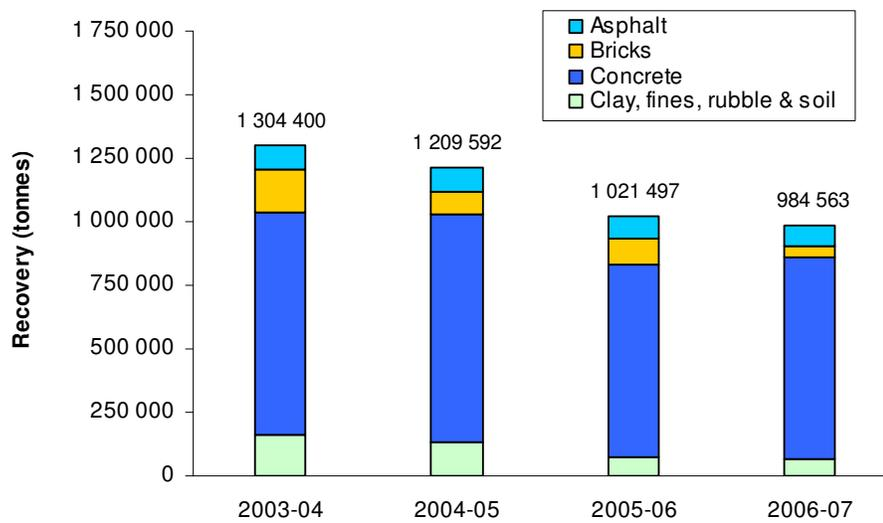
**Figure 1-6 Annual masonry materials recovery, SA 2003-04 to 2006-07**
